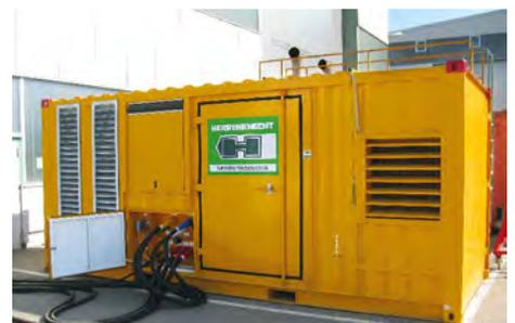
Sound isolation: power packs are installed in a sound-proofed 20 ft container.
