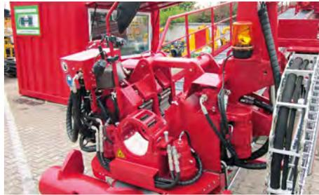
Open wrench style: allows direct access and view to the drill rod connection via mirror or camera (optional).
