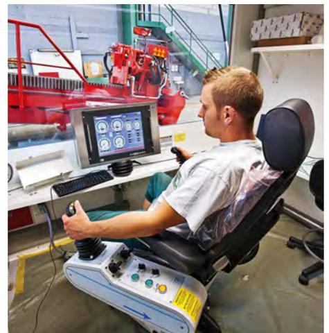
Control Cabin & Process Visualization: HDD Rig operator controls and checks the drilling process with a touch screen monitor and an ergonomic control seat with joysticks.
