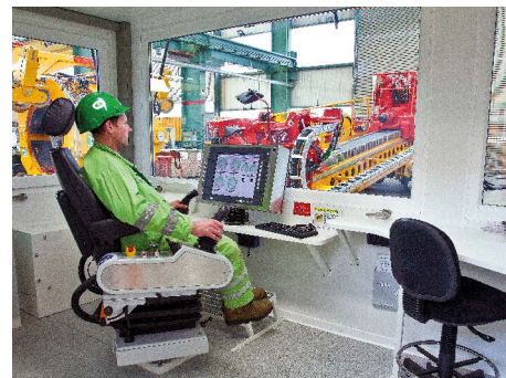
Control Cabin: ergonomic rig operator seat with joysticks, touch screen monitor and more optional indicating instruments.
