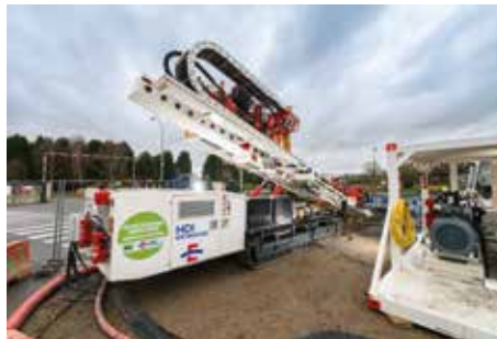
Onboard noise insulated electric power unit
