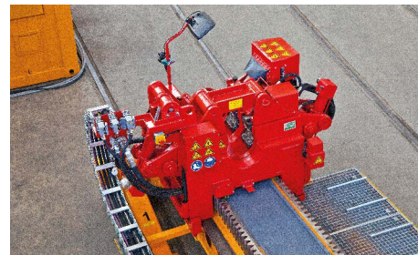
Breakout Unit: completely movable open wrench with energy chain and equipped with cameras for improved view.
