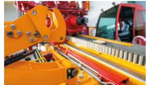
Rod loading and storage system for up to 6 drill pipes on the rig operated by the driller.
