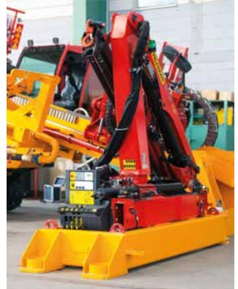
Crane connected to the front anchoring system of the HK80CK.
