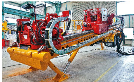
Drilling: hydraulic supports for angle adjustment of the rig.
